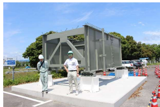
(b) End block of steel bridge
