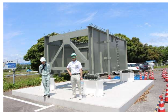
(b) End block of steel bridge
