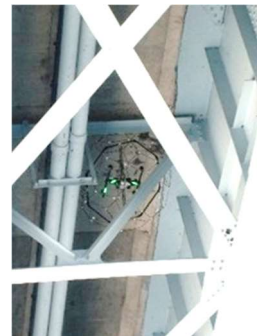
(g) Drone with rotatable spherical shell for bridge inspection
