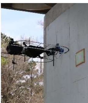
(e) Drone with hammering test equipment for bridge inspection
