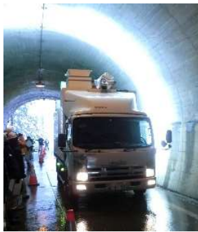
(a) Tunnel inspection system using non-contacting radar
